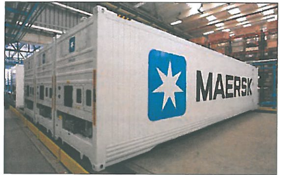
Star Cool reefers from MCI factories in China and Chile are now delivered ready to use R513A
