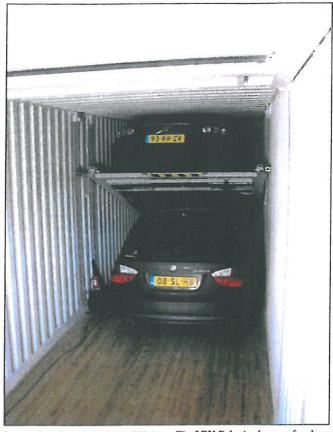
Rotterdam-based Unit45 BV is now offering automotive logistics companies in Europe a range of 45ft high-cube containers fitted with the Trans-Rak car transport system. Previously, Trans-Raks have only been installed in 40ft containers for deepsea operations.
