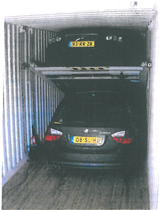
The Trans-Rak equipment is retractable, meaning containers can be used for general cargo on the return journey
